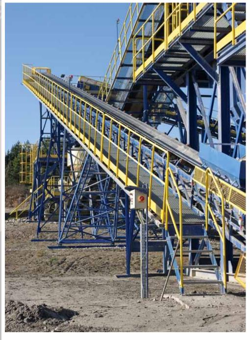
Engineered specifically for rock, our 375# and 600# belts feature a low stretch Poly / Nylon carcass, 12:1 safety factor and less than 2% stretch at full working tension. RMA grade 1 covers are included for superior cut and gouge resistance.
